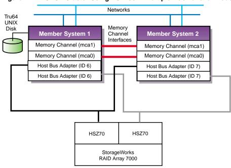
Figure 1-7: NSPOF Cluster Using HSZ70s in Multiple-Bus Failover Mode
